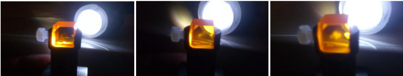
Fig. 7. Bulk damage occurring in the type-II orange phase HGS-2 OPO element generating 6.3  $\mu\text{m}$  idler pulses after using it for hours at  $>100 \text{ mJ}$  pump energy and 10 Hz.
