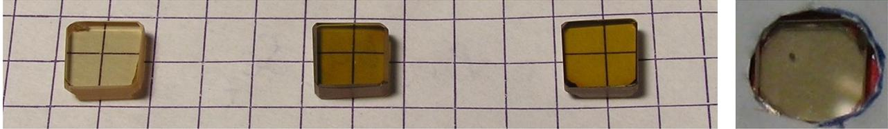
Fig. 13. Damage test plates BGS, BGSe-y, BGSe-z, and damage on test plate BGS (from left to right).
