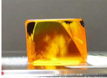
Fig. 6. Bulk damage occurring in the type-I orange phase HGS-1 OPO element generating 4  $\mu\text{m}$  idler pulses after using it for hours at  $\sim 95 \text{ mJ}$  pump energy and 100 Hz.
