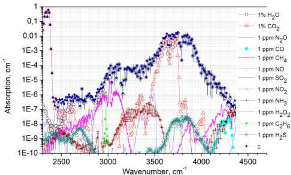
Figure 6. Absorption spectra in spectral range 2-4  $\mu\text{m}$
