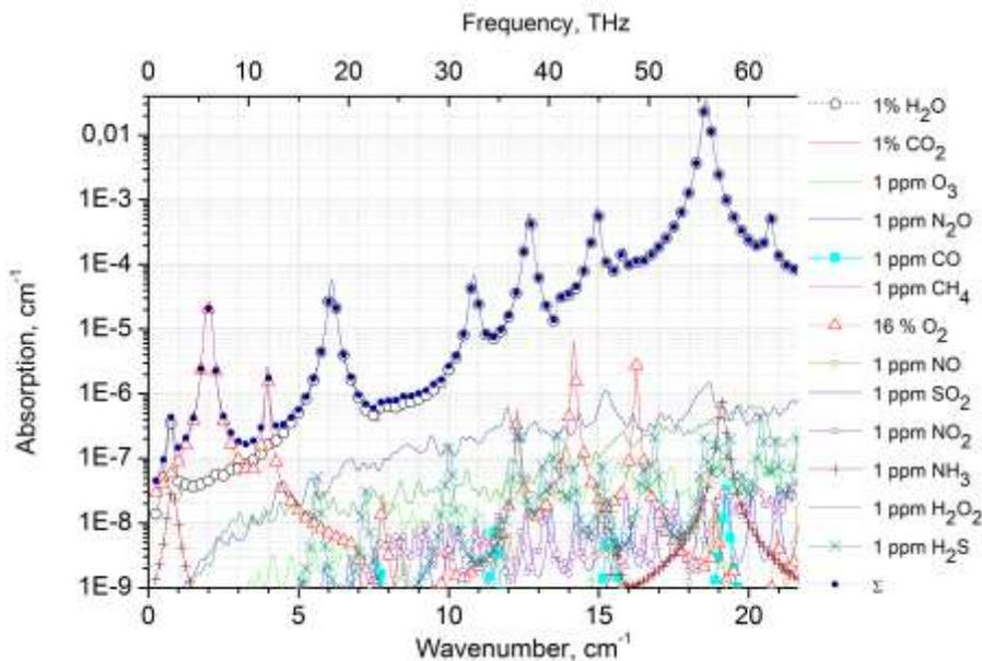
Figure 7. Absorption spectra in spectral range 2-4  $\mu\text{m}$
