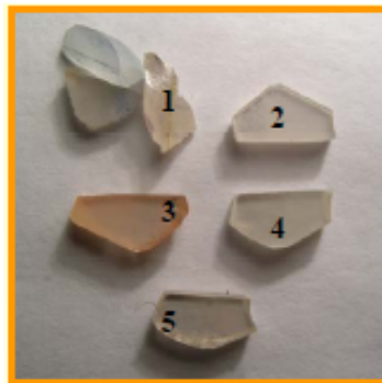
Fig. 1. LGS samples before (1) and after annealing in vacuum (2), Li 2 S (3), Ga 2 S 3 (4) and S (5).
